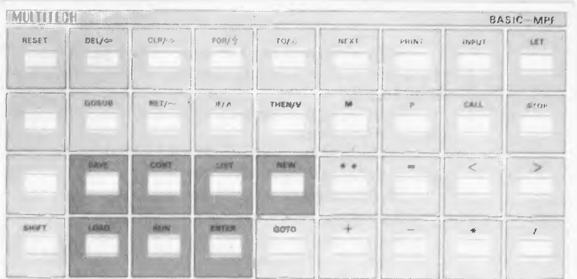
Pictured here are the Micro-Professor keyboard overlays. They fit neatly over the standard keyboard to alter the function of each key.
